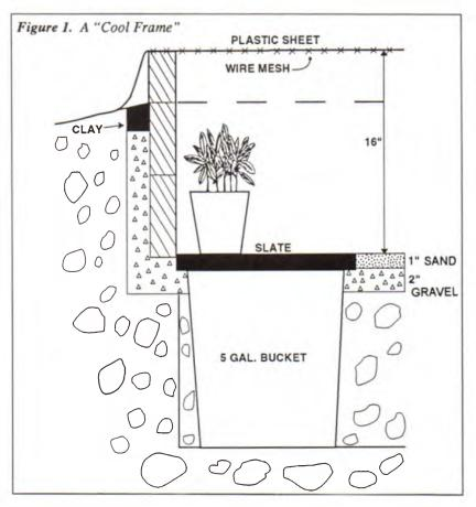
lower frames or walls. The four-inch side of the 2" x 4"'s makes the vertical side of the frame. Then 2" x 4" heavy wire mesh is nailed across the wood frame. Keep the wire mesh pulled tightly as it is nailed onto the top of the frame. Nails are driven one-half into the wood and then bent over to secure the wire in place. Any excess wire is cut off or bent over the edge of the frame.
