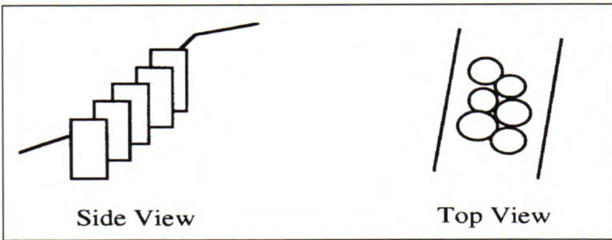
Using tree-trunk sections to build hillside steps
